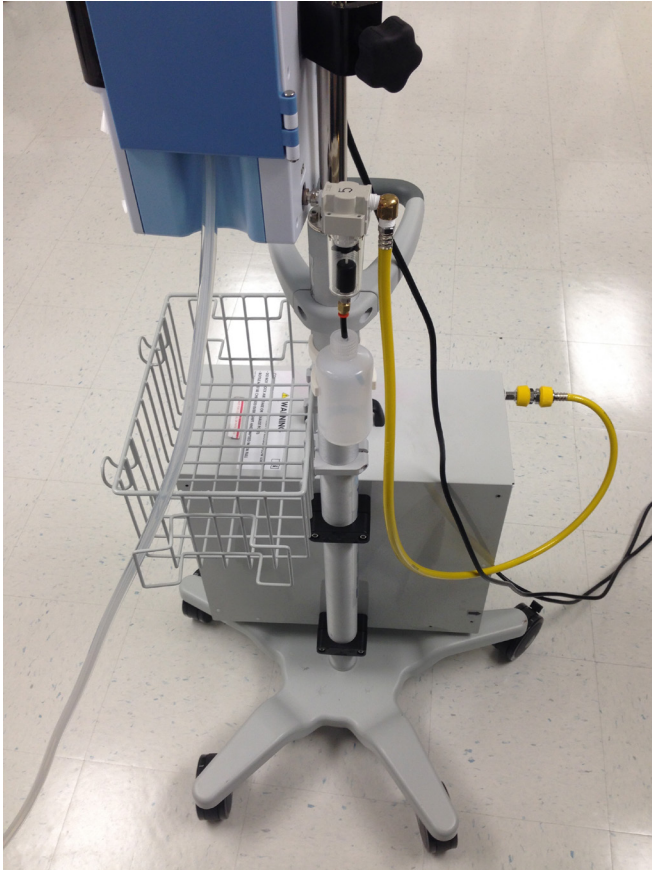
The Precision Flow with High Altitude High Flow Kit, fully assembled.
