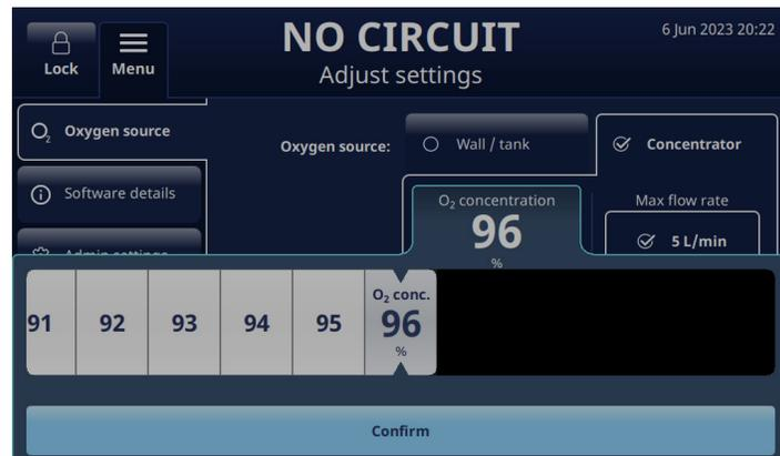
Figure 15: **Concentrator** - Scroll bar to change O<sub>2</sub> changes
