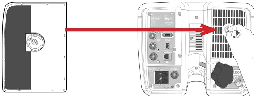
Figure 48: Insert the patient air intake filter into the back of the device
