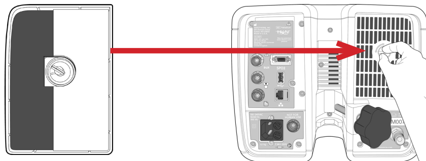
Figure 53: Insert the patient air intake filter into the back of the device
