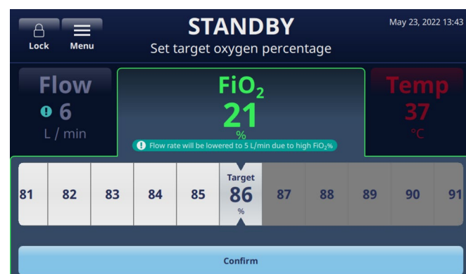
Figure 45: Screen messages providing high flow rate guidelines
