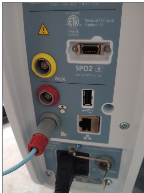
Figure B1: HVT 2.0 EMR Link cable placed in the EMR data port
