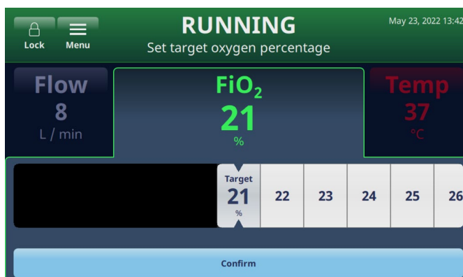
Figure 29: Setting the FiO 2 parameter using the scroll bar
