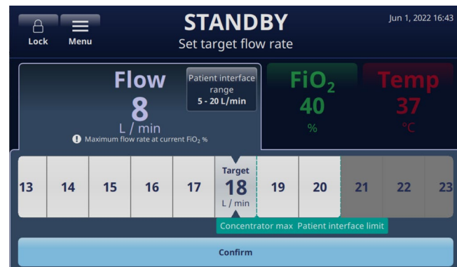
Figure 32: Notification of changes in FiO 2 as flow rate changes
