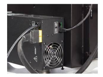
24. Remove the grey communication cable from the package and insert it into the inverter. The cable should be inserted into the receptacle labeled **COMM1 GREY.**
