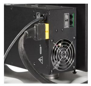
23. Remove the black communication cable from the package and insert it into the inverter. The cable should be inserted into the receptacle labeled **COMM2 BLACK.**
