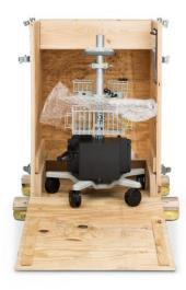
7. Unlock the VTU wheels and roll the VTU out of the crate.
