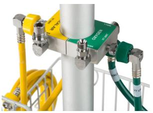
18. Attach the 3-foot air hose labeled **TANK** to the corresponding connection port on the air manifold also labeled **TANK**.
